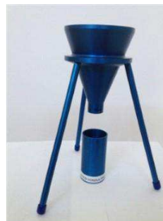
Funnel, Pourability and Bulk Density Cup, 10mm, KC800810
